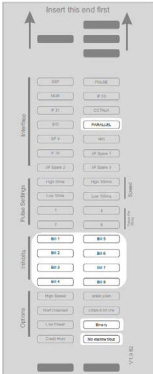
When using the configuration card to set parallel mode, the following options are available:
