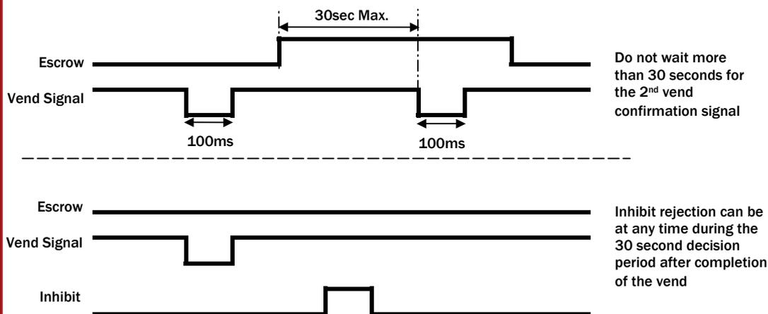
Figure 15 - Escrow Timing Diagram for Parallel Vends
