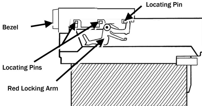
Figure 10 - Bezel and NV9 USB Installation
