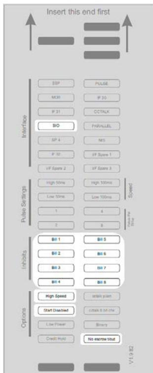
When using the configuration card to set SIO mode, the following options are available:
