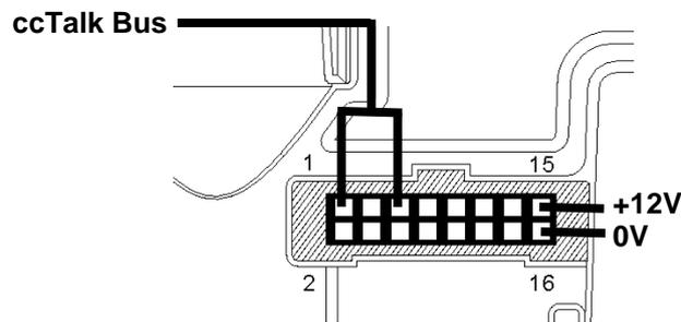
Figure 4 - ccTalk pin connection diagram
