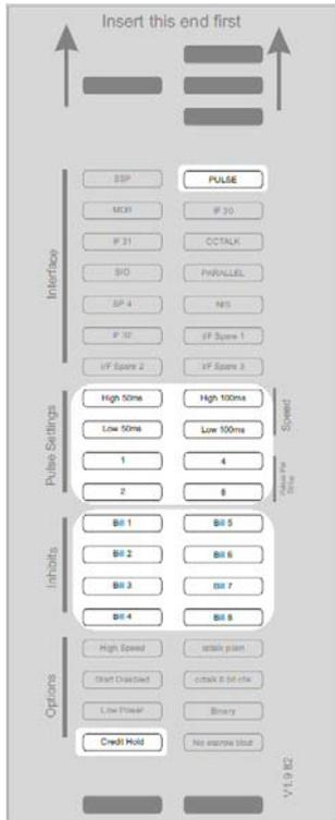
When using the configuration card to set pulse mode, the following options are available:
